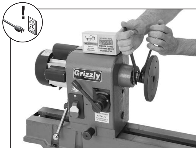
Figure 26. Tightening the faceplate onto the spindle.
